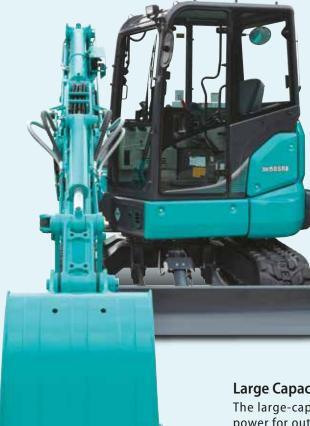
**Easy Hydraulic Piping for Quick** Hitch (Option) Piping for guick Hitch is useful for changing attachment.
