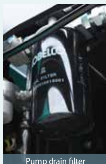
Pump drain filter
