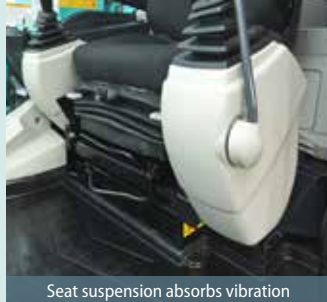
Seat suspension absorbs vibration
