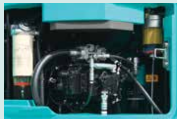
Fuel filter with built-in water-separator
