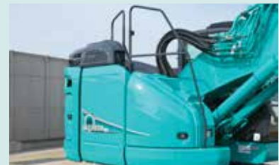
Handrail The handrail on the step side allows easy access to the maintenance port on the upper arm.
