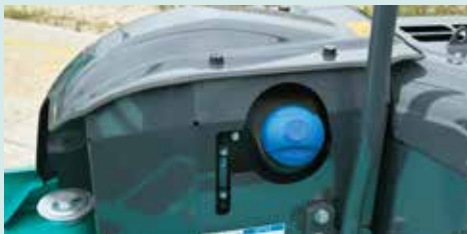
Urea tank Urea filler cap is placed on the step for easy access.
