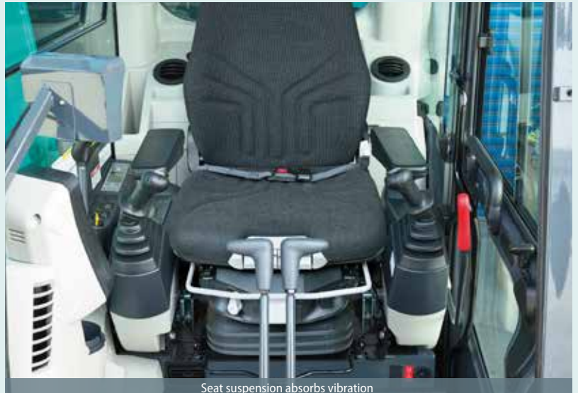
Seat suspension absorbs vibration
