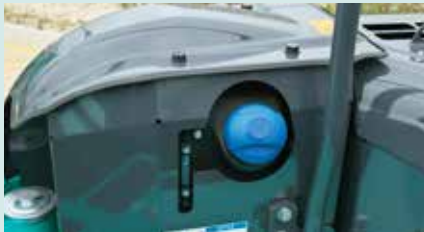
Urea tank Urea filler cap is placed on the step for easy access.
