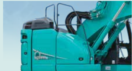
Handrail The handrail on the step side allows easy access to the maintenance port on the upper arm.
