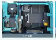
Laid out for easy access to radiator and cooling system elements
