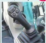
It takes 25% less effort to work the operation lever, which reduces fatigue over long working hours or continued operations.
