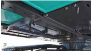
Frame is reinforced from the factory to support the heavier counterweight.
