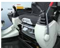
Suspension seat absorbs vibration
