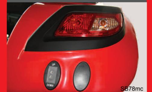
The 3-point lift arm control buttons are positioned on the rear fender under the rear light.
