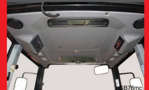
Nicely finished, low-noise factory cabin, standard with radio and air conditioning.
