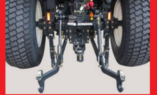
The category 1 hitch has a lift capacity of 1650 kg at the ball end.
