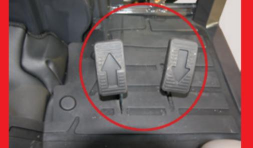
Hydrostatic control pedals for smooth hands free forward and reverse motion.
