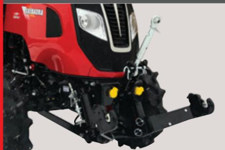
Front lift cat. 1 with a lifting capacity of 1500 kg.
