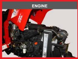
3-cylinder diesel engine delivers the highest power in its class with outstanding durability and reliability. The engines of SB22 and SB25 comply with the Stage V emission standard.
