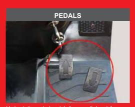
Hydrostatic control pedals for smooth handsfree forward & reverse motion (hst-models).
