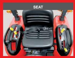
The operating levers are placed within easy reach on the left and right of the seat for ergonomic operation.
