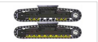
**Track guards:** to provide better protection, track alignment, and performance of machine while travelling. 2 guards per track as standard (double and full-length track guards available as options). These various track guard options provide you with optimal solutions for your extreme applications.
